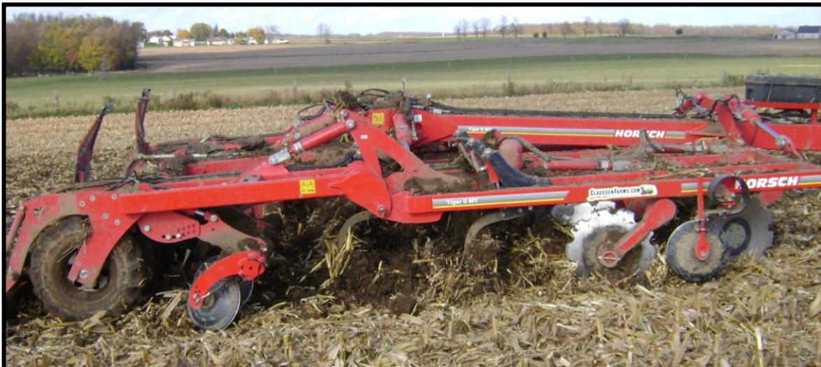
The Tiger can incorporate and blend high amounts of residue in one tillage pass and leaves the ground ready for planting with the Rapid drill. Working depth can be set between 3 and 8”.
